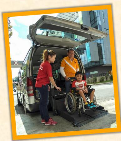
Under the year of review, we saw the replacement of our 11-year old wheelchair accessible vehicle. The newly replaced vehicle is now incorporated with our refreshed corporate logo and colour scheme, along with a wheelchair lift of longer platform, lifting capacity and premium wheelchair securement system.
